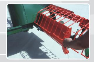
A sliding partition seals the reception chamber and speeds up the passage of grain through the auxiliary hopper.
