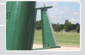
Height regulation for transport and work is set hydraulically and cylinder clamps are used to ensure steadiness in operation.
