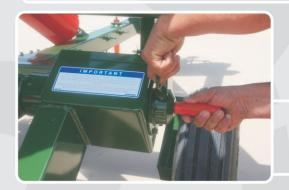
A simple pull-type locking mechanism connects and disconnects the sweeper augers in a snap.
