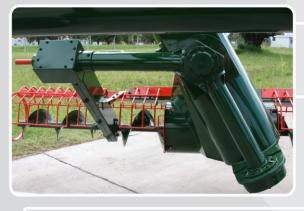
The all new auger drive is positioned away from the reception chamber to eliminate grain flow turbulence.
