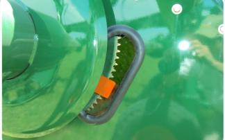
The automatic roller engage & disengage feature allows for fast release of used plastic. A marker in the viewing window notifies operator that roller drive is positively disengaged.
