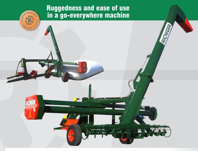
The EA-910 unloader can handle up to 12,000 bushels of corn per hour, equivalent to 300 tons/hour. Actual output will depend on grain type, moisture and degree of cleanliness.
